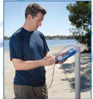
Ground water monitoring in a coastal zone using Level TROLL® 700 and RuggedReader®
