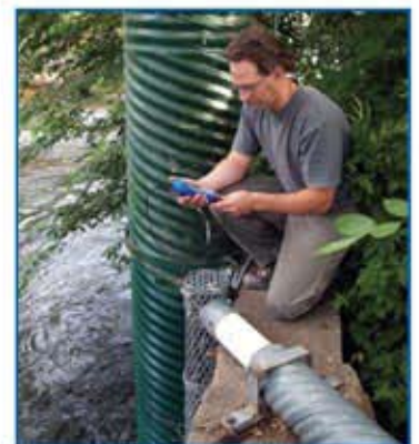
Stream gauging using Level TROLL® 500 and RuggedReader®
